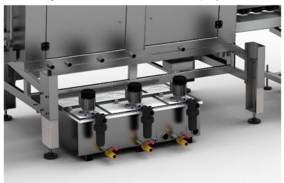
Each section is equipped with an independent water circuit, each one powered by a dedicated recirculation pump. There is a stainless-steel tank equipped with three separate sections, with cascade water flow from the last section to the first.
